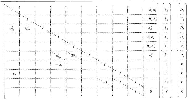
Here the subscript b denotes the booster and subscript p denotes the launch pad. Note that  $P_p$  is the generalized external force, if any, acting on the pad, such as overpressure. Again, static condensation is used to minimize the computational effort. Going through the same two-step condensation performed earlier, yields
